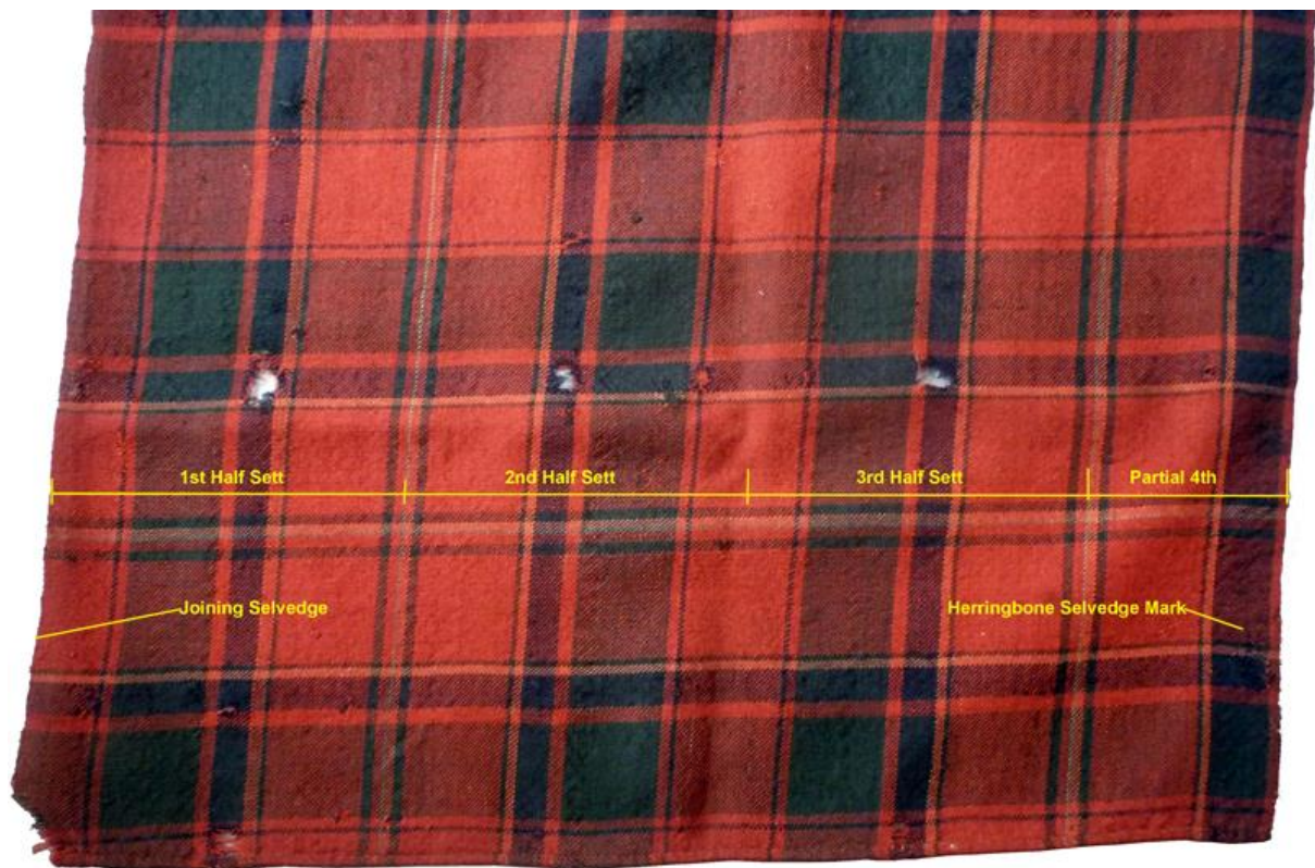
Plate 3. The off-set warp layout showing the half setts, joining and herringbone selvedges. © The Author
