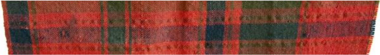
Plate. 7 Detail of the WHM specimen showing the cockling in the brown weft yarn. Photo E F Williams
